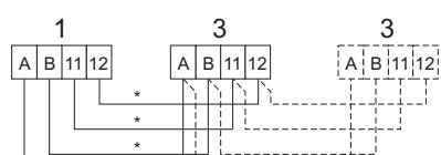
\* 4 x 0.2 mm² (AWG 24)      Serial connection
