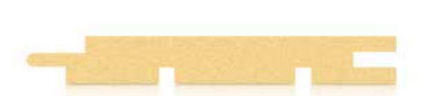
All Tylö sauna panels have the STS profile and measure 12 x 95 x 2400 mm.
